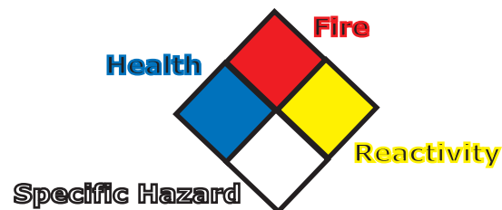
Figure 1. Hazardous Materials Identification System
